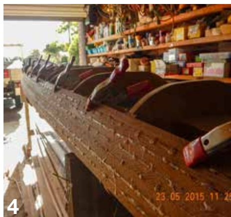
Gluing the timber strips
